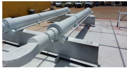
Removal of equipment, blasted and painted in workshop ready for reinstall.
