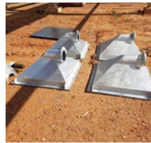
Four Pebble chutes fabricated in our workshop and installed on site.
